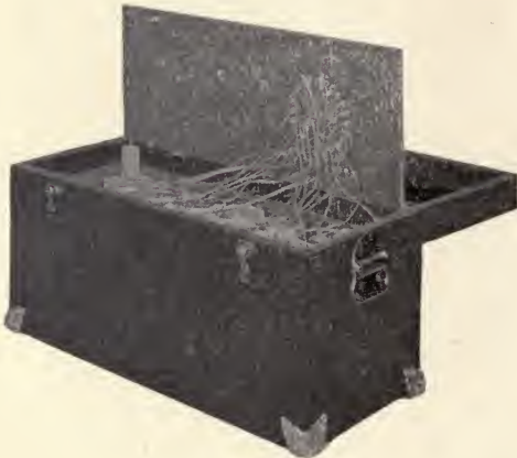
FIG. 5.—Portable Dry Cell Battery with Switchboard Raised, showing connections.
